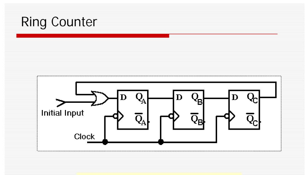
In Class: Build a ring counter using electronics simulation tools
